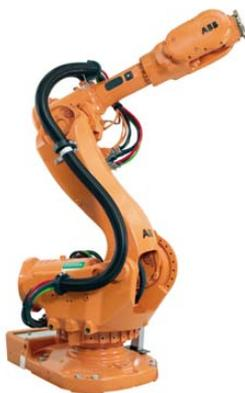
*Figure 5.2: Example of a large-size industrial robot from ABB with similar size and load capacity (175 kg) as the robot used in the experiments. Photo from ABB Robotics [2007].*
