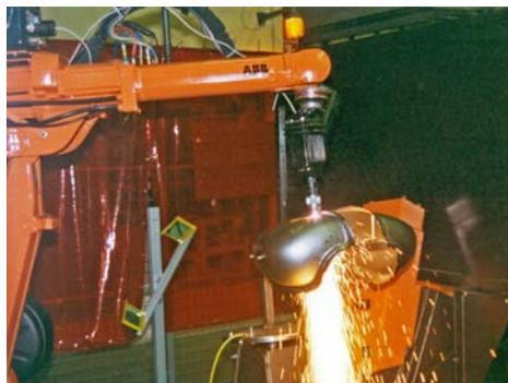
**Figure 5.1:** The industrial robot IRB1400 performing plasma cutting. The control objective is to follow a desired tool path, whereas the measured variables are the motor angular positions. The tool position and orientation are not measured due to practical and economical reasons. Photo from ABB Robotics [2007].
