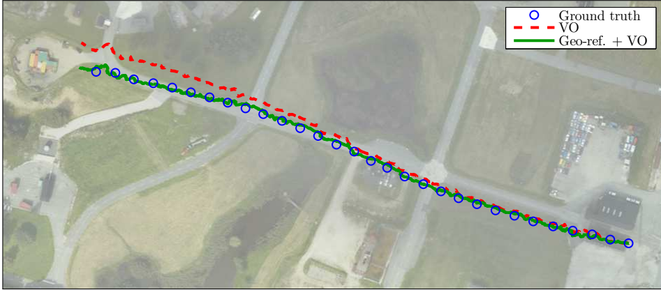
Figure 3.5: True trajectory illustrated with circles and the estimated trajectories with (solid line) and without (dashed line) geo-referencing.
