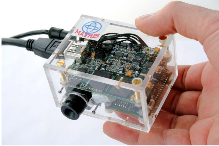
Figure 4.1: This is a prototype developed in the MATRIS project. It consists of a camera, an IMU and a low-power digital signal processor, used for pre-processing of the sensor signals. Courtesy of Xsens Technologies B.V.
