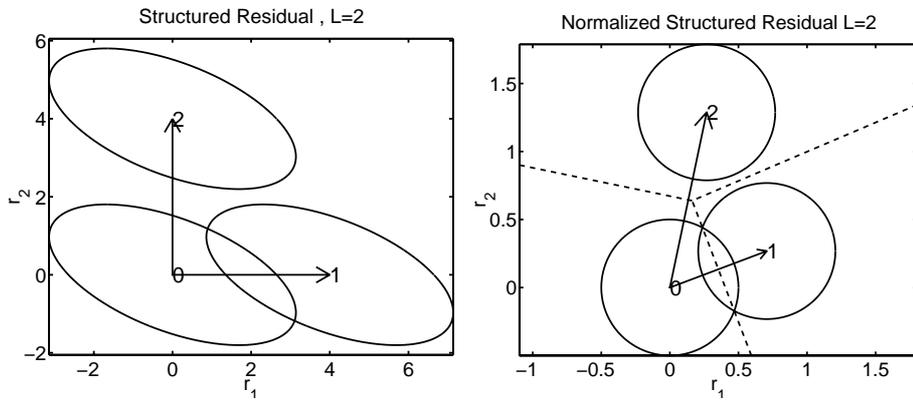
Figure 6.2: Original and normalized structured residual fault pattern with uncertainty ellipsoids for fault 1 and 2, respectively. Solid line is for unnormalized residuals, and dashed line after normalization. The dashed line is the optimal decision region.
