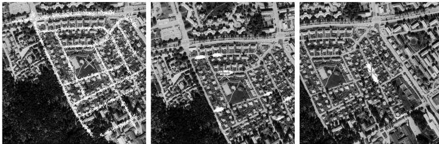
Figure 5.2: Car positioning: Sequence of illustrations of particle clouds (white dots) plotted on a flight image for visualization. The center point '+' shows the true position and 'x' the estimate.
