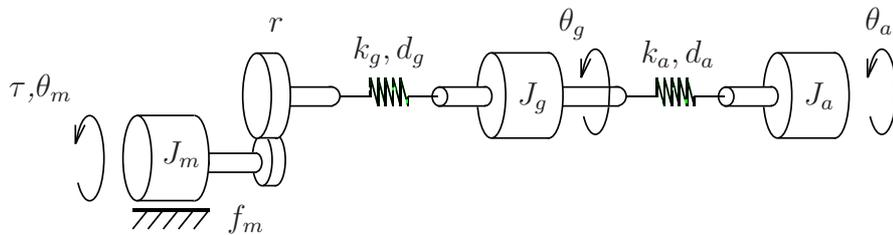
Figure 8.2: Three-mass flexible model.
