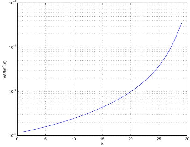
Figure 5.7: CRLB as a function of scan angle  $\alpha$ . The variance in the estimate of  $\theta$  increases when  $\alpha$  increases. In this case we have no bias.
