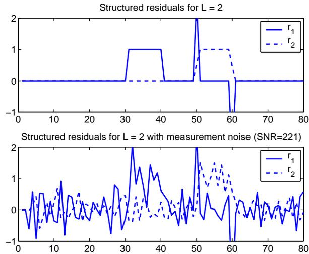
Figure 6.1: Parity space residual for a DC motor, as described in Section ??, subject to first a input voltage offset and then a sensor offset. The two residuals are designed to be non-zero for only one fault each. The lower plot illustrates extremely high sensitivity in residuals to measurement noise (SNR=221).
