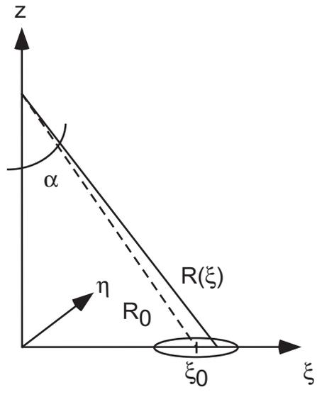
Figure 5.6: The geometry of a pulse response when the  $\eta$  axis is ignored.  $\alpha$  corresponds to the scan angle. The slant range  $\hat{R}$  is an estimate of  $R_0$ .
