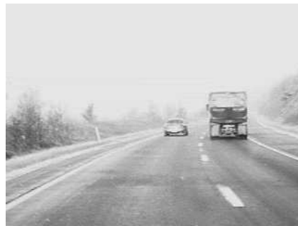
Fig. 1. When entering a curve, all vehicles start moving in the lateral direction. This information can be used to support the road geometry estimate.
