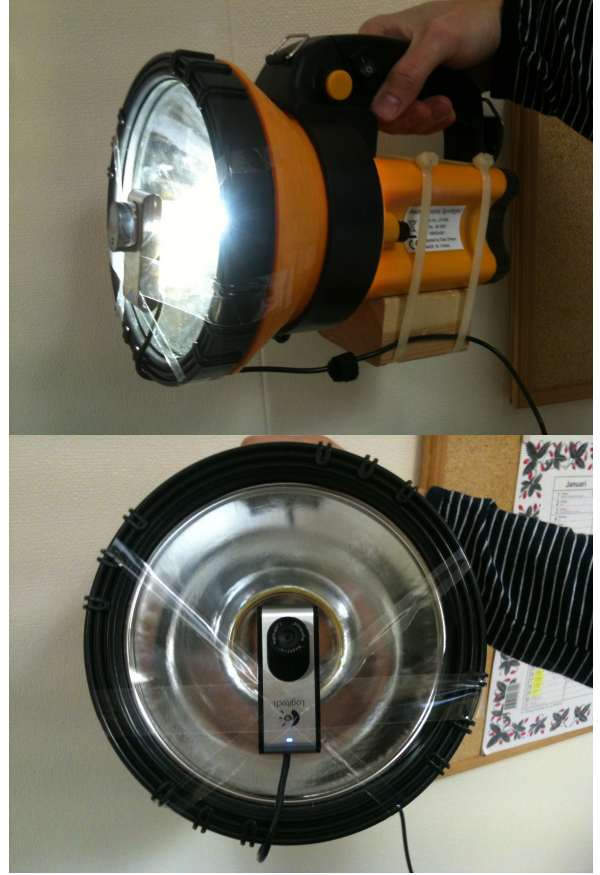
Figure 2. Experimental setup: rechargeable spotlight and a webcam glued to the center of its frontglass.
