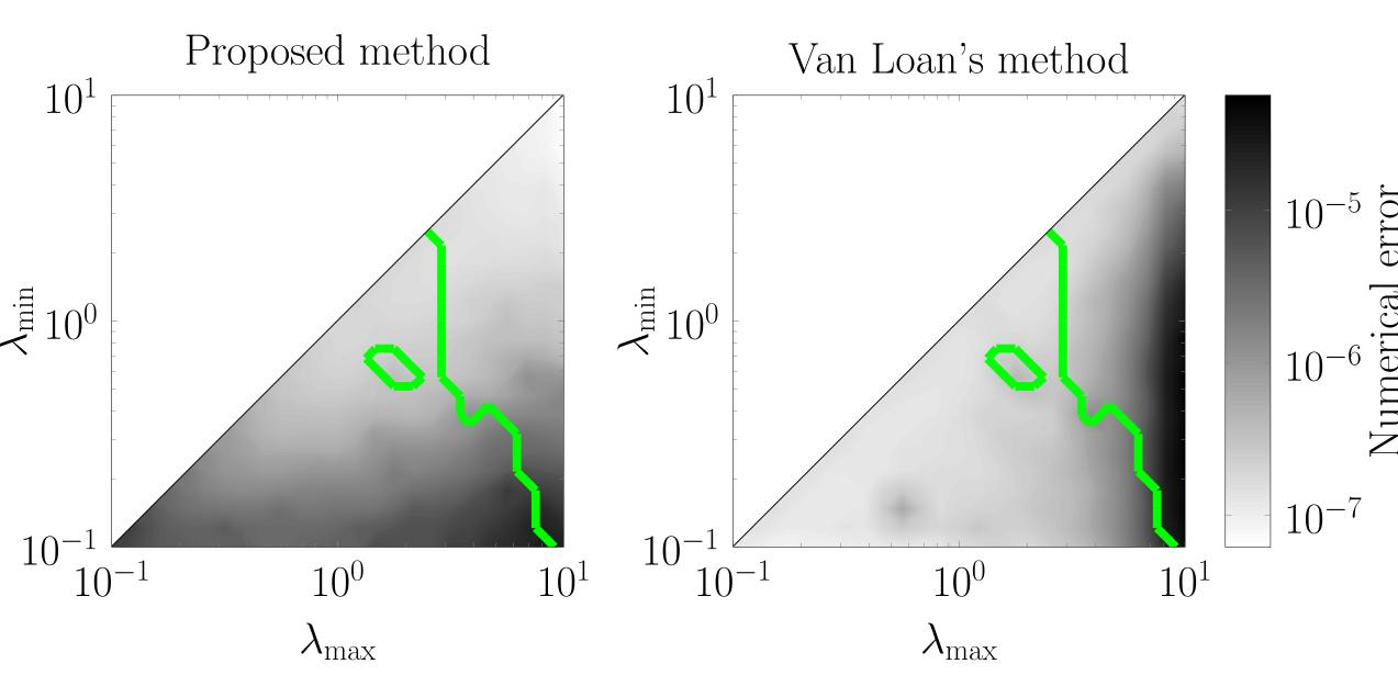
According to the results, the proposed method performs better if the slowest pole is fast and/or the sampling is slow, whereas Van Loan's method performs better if the fastest pole is slow and/or the sampling is fast. Along the green line both methods perform equally well.
