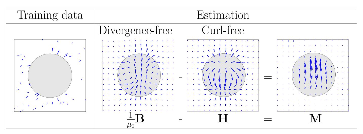
Real world data: A three-axis magnetometer has been used to measure the magnetic field at various locations around a metallic table. The position and the orientation of the magnetometer unit were measured using an optical reference system (Vicon). As a conclusion, the geometrical shape of the table could be reconstructed using these measurements.
