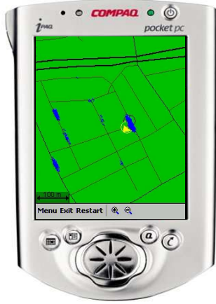
Fig. 8. Positioning without GPS, using the particle filter based on wheel speed measurements and road map only, here implemented in a handheld computer.
