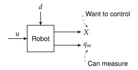
■ Want to control the TCP. Can only measure the motor angles  $q_m$ .
