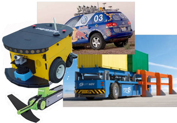
Figure 5.1: A container AGV, a robot car, an automated vacuum cleaner and a multi-purpose mobile platform illustrates the wide range of applications of mobile robots.
