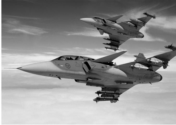
The control inputs  $u_1$  and  $u_2$  are the commanded skew- and side-rudder angles. A skew-rudder command is realized on Gripen by having the right and left hind rudders move in different directions, see Figure 1. The hind rudders are also used (together with the nose wings) to realize high altitude commands while more traditional aircrafts have separate rudders for that.
