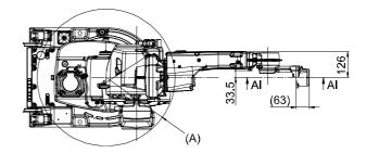
Figure 4 View of the manipulator from the back, side and above (dimensions in mm).
