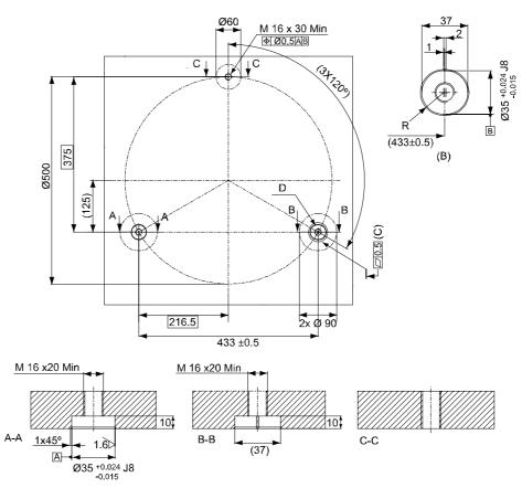
Figure 7 Mounting surface and bushings.
