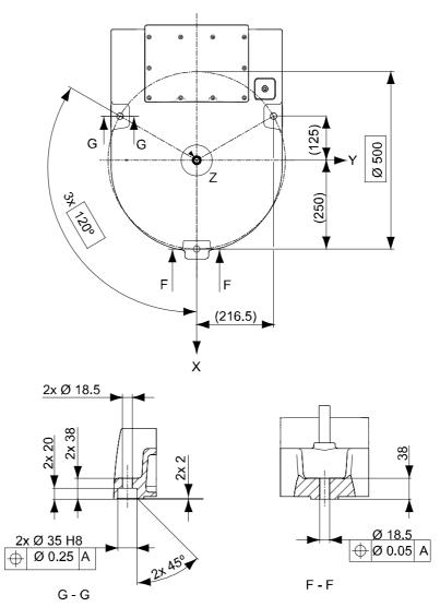
Figure 6 Hole configuration for robot base (dimensions in mm). View from the bottom of the base.
