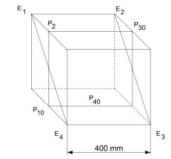
Figure 2 Path E-E2-E3-E4 in the ISO Cube, maximum load.
