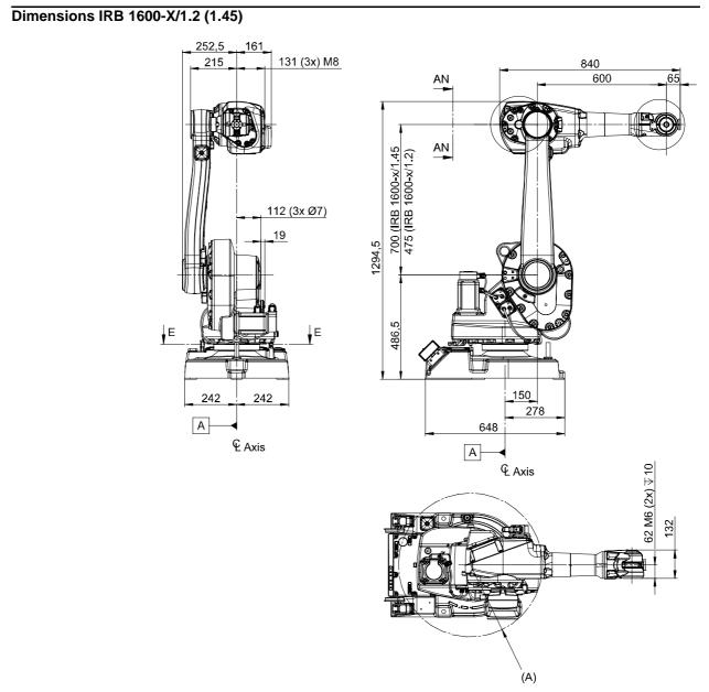
Figure 3 View of the manipulator from the back, side and above (dimensions in mm).
