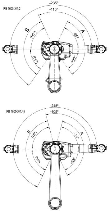
Figure 35 Mounting area of additional stop Axis 3.
