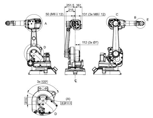
Figure 18 Holes for mounting extra equipment on the wrist, the upper arm housing and on the frame.
