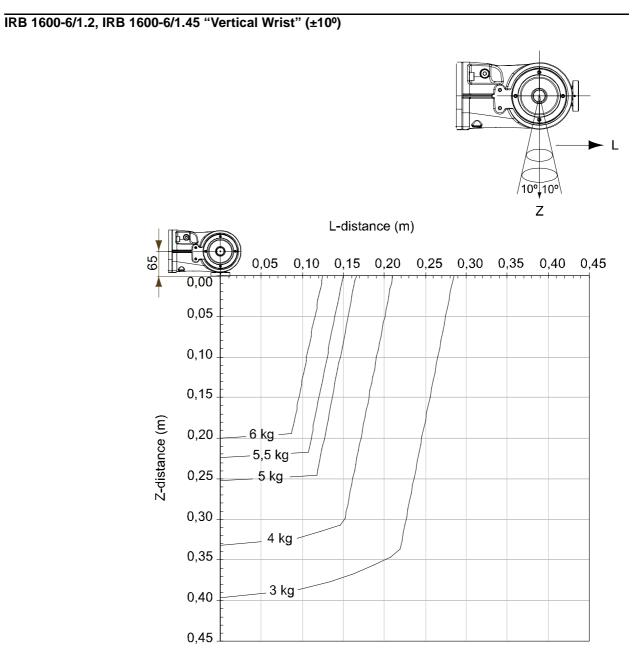
Figure 11 Maximum permitted load mounted on the robot tool flange at different positions (center of gravity) at "Vertical Wrist" ( $\pm 10^{\circ}$ ).
