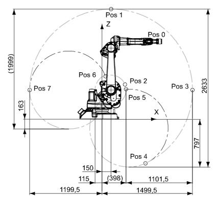
Figure 24 The extreme positions of the robot IRB 1600ID arm with 1.5 m reach.
