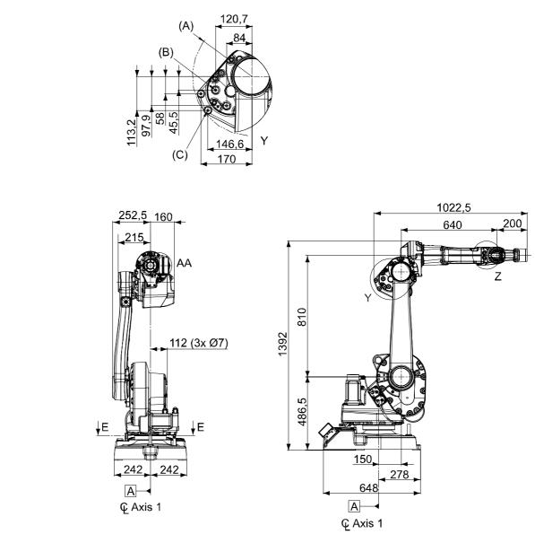
Holes for mounting of extra equipment for IRB 1600ID-4/1.5
