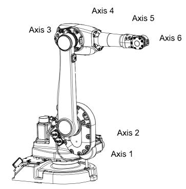
Figure 8 All axes in zero position.
