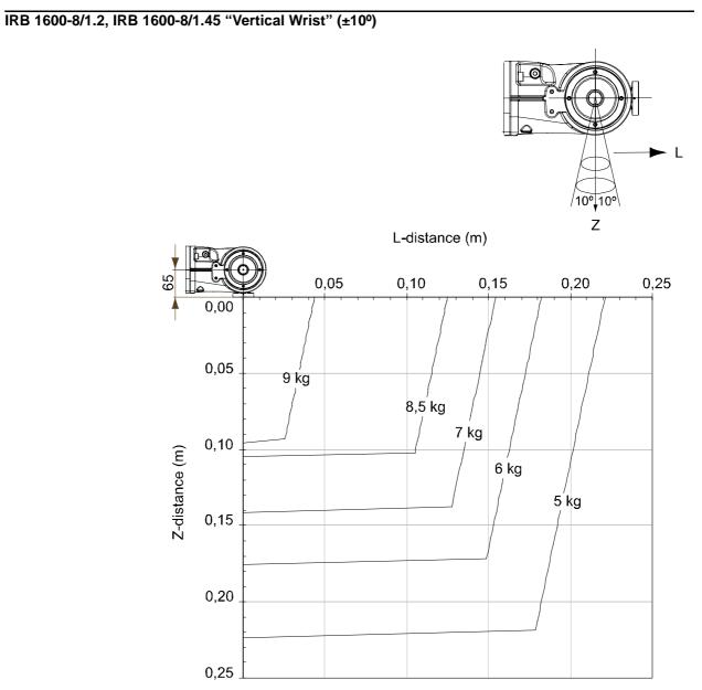
Figure 13 Maximum permitted load mounted on the robot tool flange at different positions (center of gravity) at "Vertical Wrist" (±10°).
