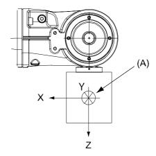
Figure 16 Moment of inertia when axis 5 center line down.
