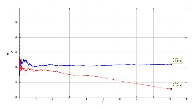
Event detection probability  $P_d$  vs time t for decaying networks with given  $P_d = 0.63$ ; with scheduling scheme (solid line) and without scheduling scheme (dashed line)
