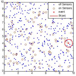
• To conserve power, sensors are switched between on state and off state
