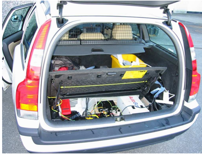
Figure 5: The collision avoidance hardware in the test vehicle.
