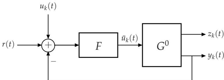
**Figure 6.3:** Closed-loop system; an example of the system description (6.1) with inputs  $r(t)$ ,  $u_k(t)$  and outputs  $y_k(t)$ ,  $z_k(t)$ . The input to  $G^0(q)$  is  $\bar{u}_k(t)$  from the controller  $F(q)$ .
