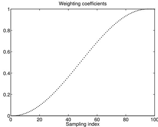
**Figure 8.8:** Coefficients for time-domain weighting of the ends of the ILC input signal.
