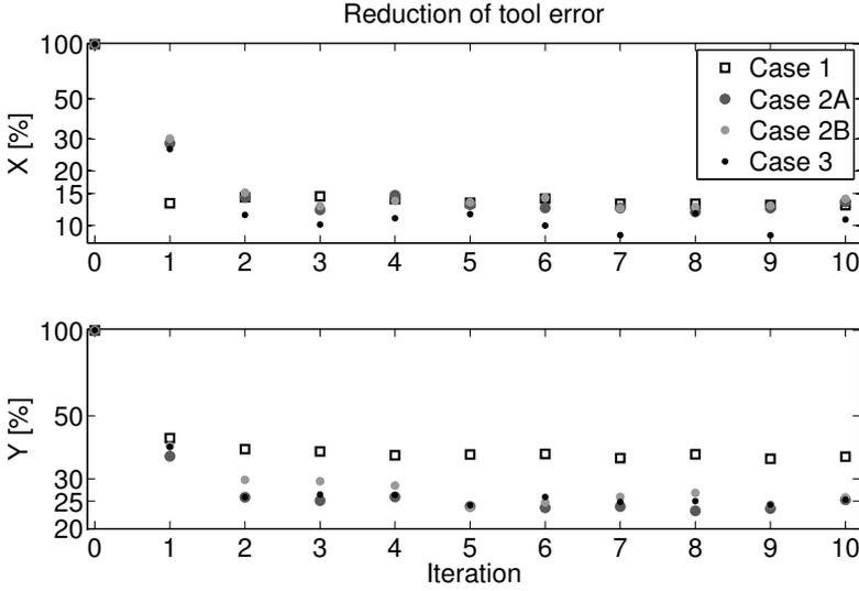
**Figure 8.13:** Comparison of error measure (8.16) of the robot tool position for the cases 1, 2A, 2B, and 3 in the X- and Y-direction, respectively..
