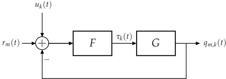
**Figure 9.1:** Simulation setup with the two-mass system represented by  $G(q)$  in discrete time. The variable  $\tau_k(t)$  denotes the motor torque from the feed-back controller  $F(q)$  at iteration  $k$ . The ILC input signal  $u_k(t)$  is added to the reference signal  $r_m(t)$  of the feedback control system. The system output in the simulation study is the motor angular position  $q_{m,k}(t)$  at iteration  $k$ .
