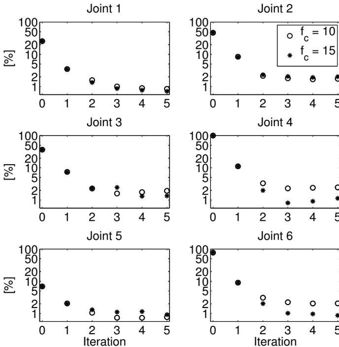
**Figure 5.8:** The error measure  $J_k^i$ , see (5.5), expressed in  $\infty$ -norm for all joints  $i = 1, \dots, 6$ , cutoff frequencies  $f_c = 10$  and 15 Hz for each iteration. A higher cutoff frequency gives a larger reduction of the errors.
