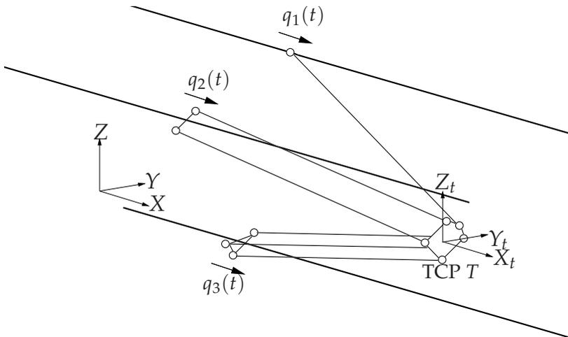
**Figure 8.1:** Schematic picture of the Gantry-Tau parallel robot, with the base coordinate frame  $XYZ$ , the coordinate frame  $X_t Y_t Z_t$  of the end-effector plate and the tool position  $T$ . Three carts move on guideways. The corresponding cart positions are denoted  $q_1(t)$ ,  $q_2(t)$  and  $q_3(t)$ .
