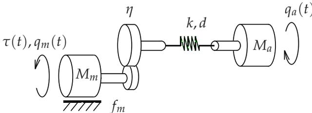
**Figure 2.4:** A two-mass model of the dynamics of a single robot joint. It is characterised by spring coefficient  $k$ , damping coefficient  $d$ , viscous friction  $f_m$ , gear ratio  $\eta$ , moments of inertia  $M_m$ ,  $M_a$ , motor angular position  $q_m$  and joint angular position  $q_a$ . The motor torque  $\tau$  is generated by a torque constant  $k_\tau$  times the input voltage.
