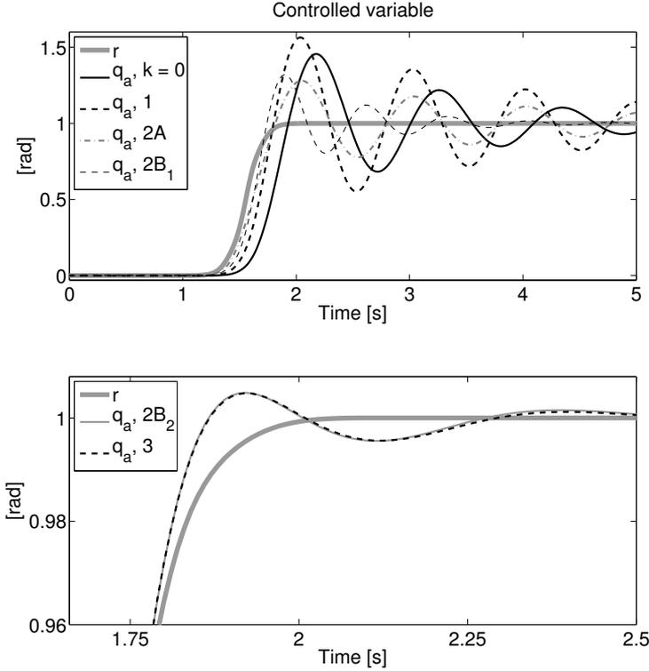
**Figure 6.7:** Actual joint angular position  $q_a(t)$  after 1000 iterations for the cases 1 to 2B<sub>1</sub> compared to the joint angular position when no ILC algorithm is applied (denoted  $k = 0$ ) in the upper figure. The lower figure shows  $q_a(t)$  after 1000 iterations for the cases 2B<sub>2</sub> and 3. Note the different axes in the figures. The performance highly depends on the quality of the estimate  $\hat{q}_a(t)$ .
