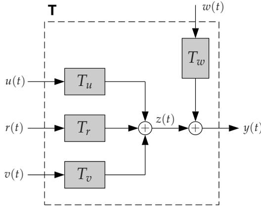
**Figure 4.1:** Representation of the system used for analysis of ILC. Inputs are the reference signal  $r(t)$ , an externally generated ILC control signal  $u(t)$ , and load and measurement disturbances  $v(t)$  and  $w(t)$ , respectively. Controlled output is  $z(t)$  and measured output is  $y(t)$ . The system  $T$  contains the system to be controlled as well as the controller in operation.
