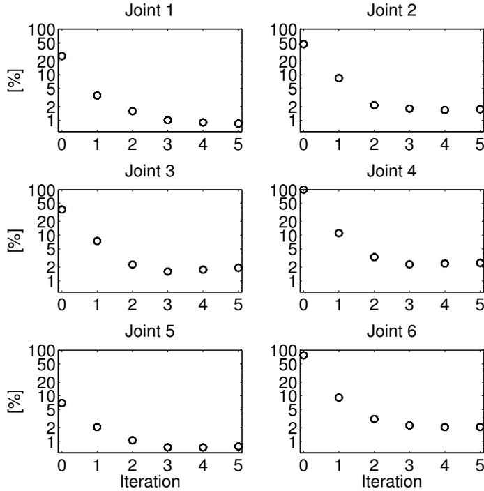
**Figure 5.5:** The error measure  $J_k^i$ , see (5.5), expressed in  $\infty$ -norm for all joints  $i = 1, \dots, 6$  for each iteration. The experiment is performed with the ILC design variable  $f_c = 10$  Hz and shows an improved performance for all joints. Note the logarithmic scale.
