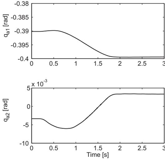
**Figure 7.3:** The desired tool motion is half a circle, with the resulting joint angular positions  $q_{a1}(t)$  and  $q_{a2}(t)$  shown in the figure.
