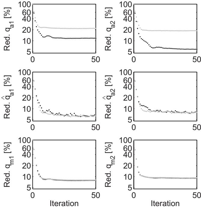
**Figure 7.8:** Case 2A: Error measure (7.9) in 2-norm as a function of iteration number for the motor and joint angular position errors, for the case with nominal system parameters (black) and the system with model errors (grey).
