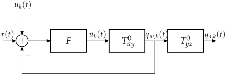
**Figure 6.5:** The two-mass system illustrated by  $T_{u_y}^0(q)$  and  $T_{y_z}^0(q)$ ; transfer function from motor torque  $\bar{u}_k(t)$  to motor angular position  $q_{m,k}(t)$  and from motor angular position  $q_{m,k}(t)$  to joint angular position  $q_{a,k}(t)$ , respectively. The system is controlled by the feedback controller  $F(q)$ , and the ILC input  $u_k(t)$  added to the reference  $r(t)$  at iteration  $k$ .
