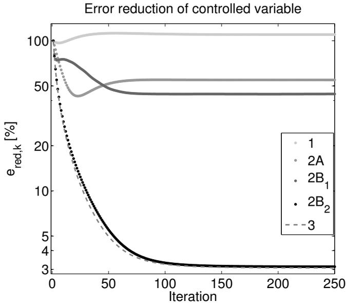
**Figure 6.6:** Reduction of  $e_k$  given by (6.36) for the first 250 iterations for the cases 1 to 3. The error reduction highly depends on the quality of the estimate  $\hat{q}_{a,k}$ .
