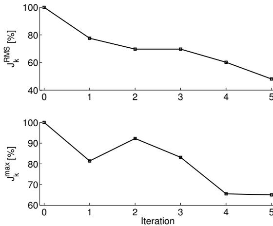
**Figure 5.6:** Tool-position error evaluated by  $J_k^{RMS}$  from (5.8), and  $J_k^{max}$  from (5.9), for each iteration. In the experiment the ILC design variable is  $f_c = 10$  Hz.
