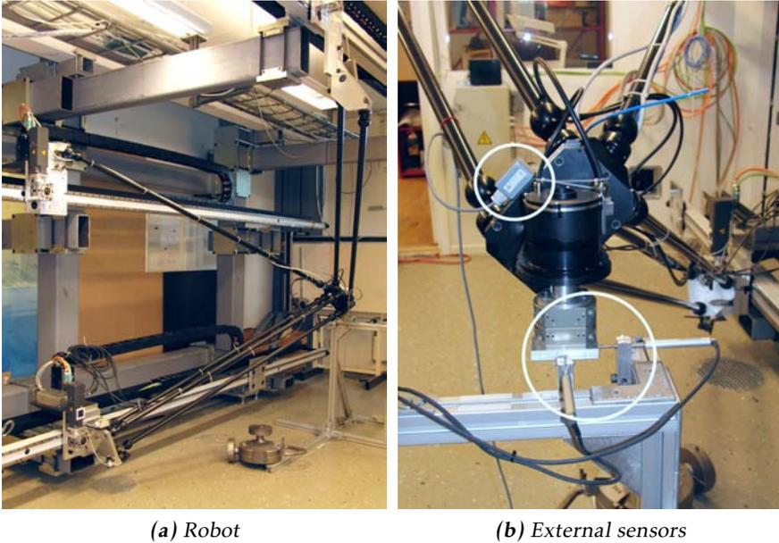
**Figure 8.2:** Experimental setup of the Gantry-Tau robot; a) robot structure, b) mounting of length gauges and accelerometer.
