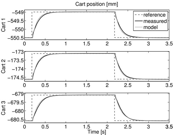
**Figure 8.7:** Model validation of the cart positions. Output (model) from the motor models (8.2) for the three carts, validated using data (measured) from the step-response experiments.
