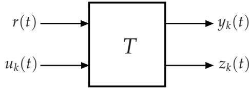
**Figure 6.1:** Description of the system  $T$  with reference  $r(t)$ , ILC input  $u_k(t)$ , measured variable  $y_k(t)$  and controlled variable  $z_k(t)$  at iteration  $k$ .
