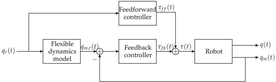
Figure 2.7: Block diagram of the robot motion control.
