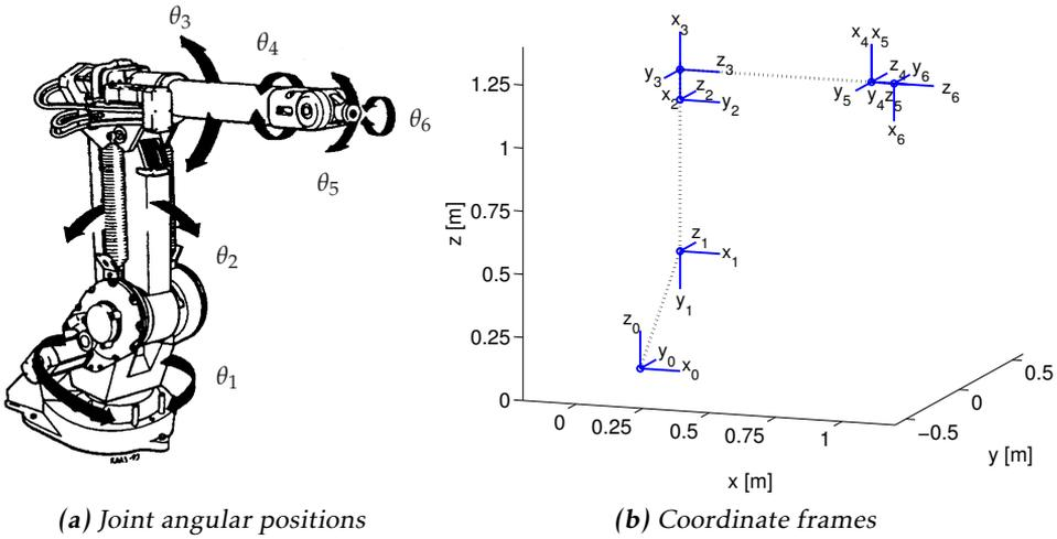
**Figure 2.2:** The ABB robot IRB1400 with a) joint angular positions  $\theta_i$ ,  $i = 1, \dots, 6$  and b) coordinate frames for each joint of the robot.
