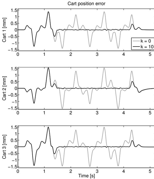
**Figure 5.13:** Cart position errors after 10 iterations compared to the nominal errors for the three carts. The errors for the part of the trajectory to be learned ( $t = 1.6 - 4.1$  s) are significantly reduced.
