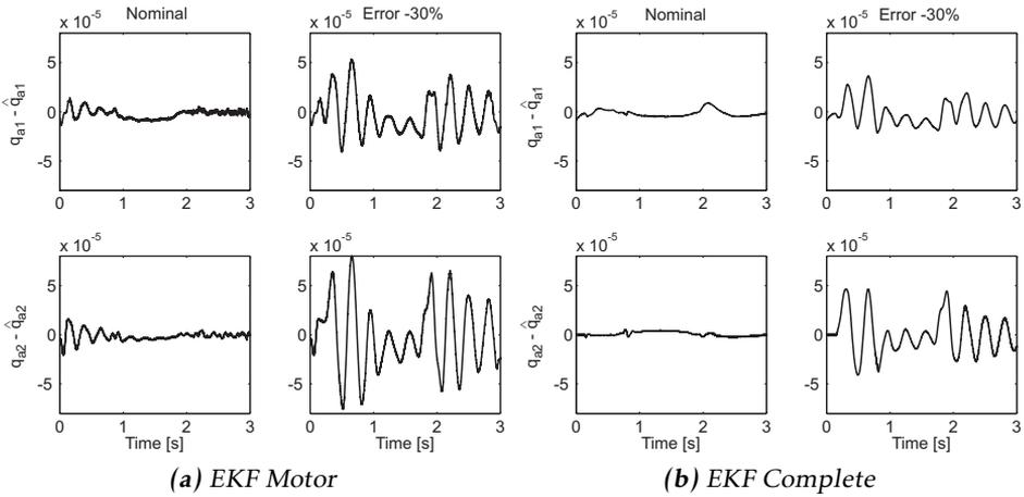
**Figure 7.4:** The estimation error  $q_a(t) - \hat{q}_a(t)$  shown for the two joint angular positions for the case with nominal parameters and modified joint stiffness parameters by  $-30\%$ . a) EKF based on motor angular position measurements (EKF Motor). b) EKF based on measurements of motor angular position and tool acceleration (EKF Complete).
