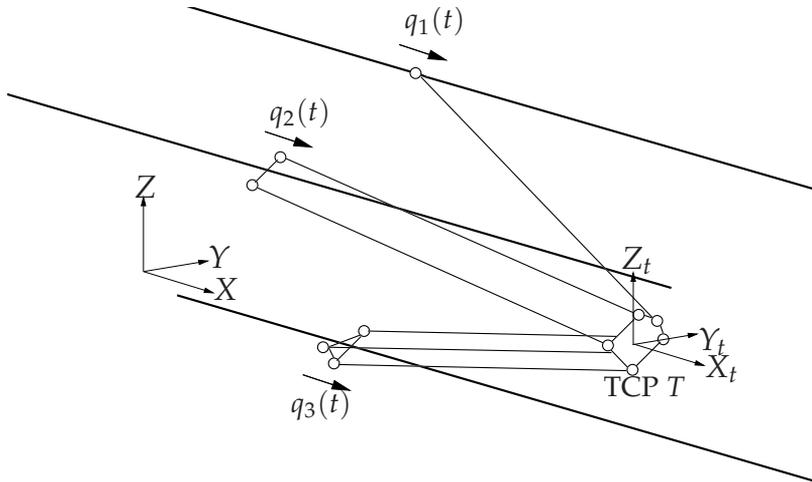
**Figure 5.11:** Schematic picture of the Gantry-Tau parallel robot, with the base coordinate frame  $XYZ$ , the coordinate frame  $X_t Y_t Z_t$  of the end-effector plate and the tool position  $T$ . Three carts move on guideways. The corresponding cart positions are denoted  $q_1(t)$ ,  $q_2(t)$  and  $q_3(t)$ .
