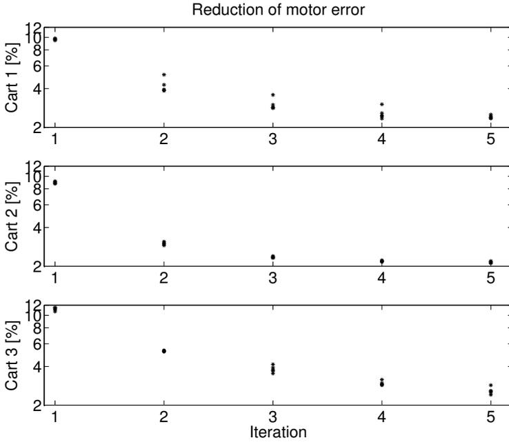
**Figure 8.10:** Case 1: Error measure (8.15) for each cart when performing five experiments with identical ILC input signal at first iteration.
