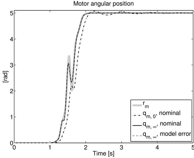
**Figure 5.17:** Resulting motor angular position when the ILC algorithm has converged (denoted  $\infty$ ). The performance is improved both in the nominal case and the case with model error, compared to when no ILC algorithm is applied (denoted 0).
