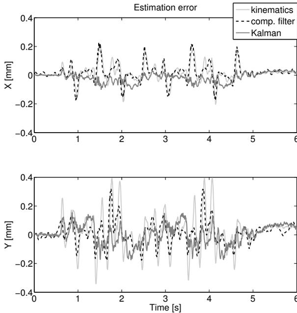
**Figure 8.9:** Estimation error  $e(t) = z(t) - \hat{z}(t)$  for the rectangular motion. Result for the calculated tool position  $z_c(t)$  from motor angular positions transformed by the forward kinematics (kinematics) compared to results from the complementary filter (comp. filter) and the Kalman filter (Kalman).
