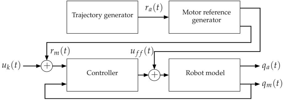
**Figure 7.2:** The robot system used in the simulation. The motor angular position reference  $r_m(t)$  is computed using the kinematic and dynamic models. The robot model is controlled by independent joint control, represented by the controller block, and by a model-based feedforward term  $u_{ff}(t)$ . The ILC input signal  $u_k(t)$  at iteration  $k$  is added to  $r_m(t)$ .
