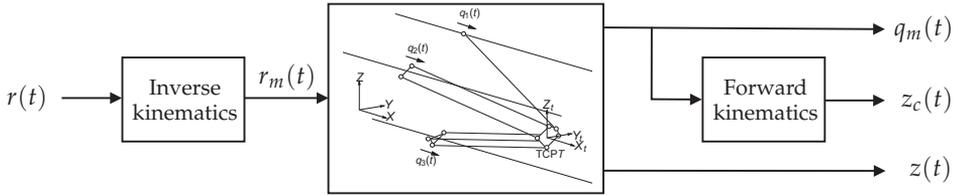
**Figure 8.5:** Robot system with signals used in the identification. The motor angular position reference  $r_m(t)$  is derived from the tool-position reference  $r(t)$  using the inverse kinematics. A calculated tool position  $z_c(t)$  is derived from measured motor angular position  $q_m(t)$  transformed by the forward kinematics. The measured tool position is denoted  $z(t)$ .
