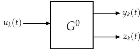
**Figure 6.2:** Stable open-loop system; an example of the system description (6.1) with input  $u_k(t)$  and outputs  $y_k(t)$  and  $z_k(t)$ .
