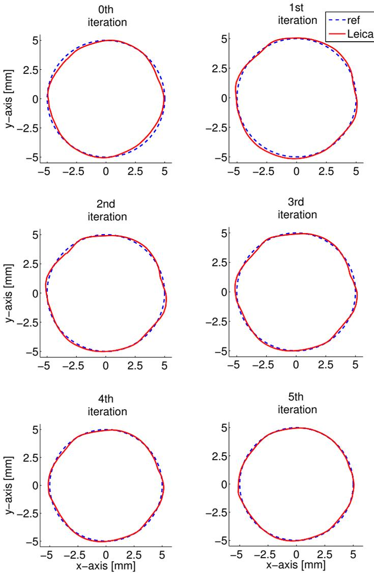
**Figure 5.7:** Measured circles of the tool at every iteration, compared to the reference circle. The experiment is performed with ILC design variable  $f_c = 10$  Hz. After five iterations the measured circle is close to the reference.
