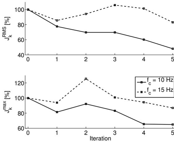
**Figure 5.9:** Tool-position error evaluated by  $J_k^{RMS}$  from (5.8), and  $J_k^{max}$  from (5.9), for each iteration. Higher cutoff frequency  $f_c$  gives larger errors.
