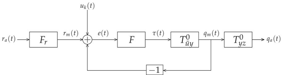
**Figure 5.16:** The system illustrated by the true systems  $T_{uy}^0$  and  $T_{yz}^0$ , relating motor torque  $\tau(t)$  to motor angular position  $q_m(t)$ , and motor angular position  $q_m(t)$  to joint angular position  $q_a(t)$ , respectively.  $F$  represents the controller. The reference  $r_a(t)$  is filtered by the pre-filter  $F_r$ , giving  $r_m(t)$ , and the ILC input  $u_k(t)$  is added to  $r_m(t)$ .
