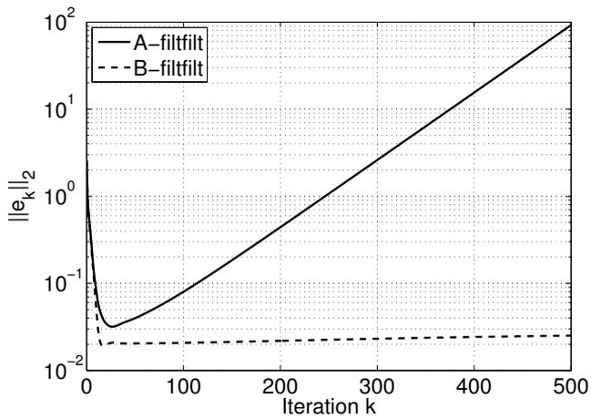
**Figure 9.6:** 2-norm of the error as function of iteration index when the filter form (9.33) of the ILC algorithm is used for the cases A and B together with the *filtfilt* command.
