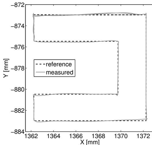
**Figure 8.12:** Case 2A: Tool performance after 10 iterations, with reference path compared to measured tool path.
