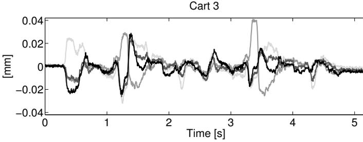
**Figure 8.4:** The difference (8.1) for cart 3, for five identical experiments illustrates the repeatability of the system.
