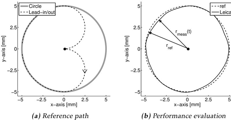
**Figure 5.4:** a) Reference path for the robot tool position with lead-in/lead-out, b) performance evaluated on the circular path, see (5.6) to (5.7).
