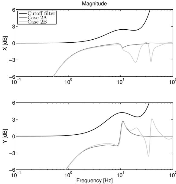
**Figure 8.11:** Case 2A, 2B: The magnitude  $|\bar{Q}^{-1}(e^{i\omega T_s})|$  of the filter  $\bar{Q}(q)$  cutting off the learning over about 30 Hz illustrated together with the magnitude  $|1 - L(e^{i\omega T_s})(F_u(e^{i\omega T_s}) + F_y(e^{i\omega T_s})T_{uy}(e^{i\omega T_s}))|$  in the  $X$ - and  $Y$ -direction.
