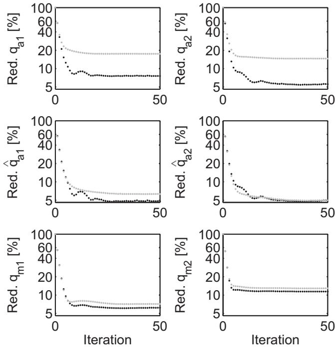
**Figure 7.9:** Case 2B: Error measure (7.9) as a function of iteration number for the motor and joint angular position errors for the case with nominal system parameters (black) and the system with model errors (grey).
