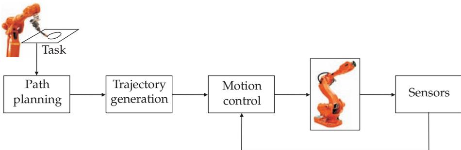
*Figure 2.6: Block diagram of the robot control system.*
