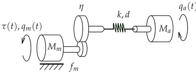
**Figure 5.15:** A flexible two-mass model characterised by spring coefficient  $k$ , damping coefficient  $d$ , viscous friction  $f_m$ , gear ratio  $\eta$ , moments of inertia  $M_m$ ,  $M_a$ , motor angular position  $q_m(t)$ , joint angular position  $q_a(t)$  and motor torque  $\tau(t)$ , generated by a torque constant  $k_\tau$  times the input voltage.
