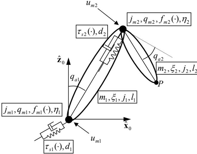
**Figure 7.1:** The two-link robot model used in the simulation. The rigid links are described by mass  $m$ , link length  $l$ , center of mass  $\xi$  and inertia  $j$  with respect to the center of mass. The elastic joints are described by gear ratio  $\eta$ , nonlinear spring torque  $\tau_s$  and linear damping  $d$ . The nonlinear friction torque  $f$  acts on the motors. The deflection in each joint is described by the motor angular position  $q_m$  and joint angular position  $q_a$ .
