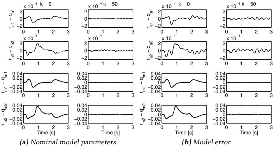
**Figure 7.5:** Case 1: Resulting motor and joint angular position errors for ILC iteration  $k = 50$ , compared to the errors when no ILC algorithm is applied to the system (denoted  $k = 0$ ). a) nominal system parameters, b) model errors introduced. The error reduction is smaller for the case with model errors, as expected. The different scaling for motor angular position and joint angular position is due to the gear ratio  $\eta = 200$ .
