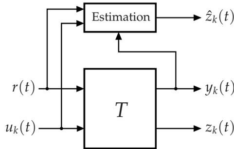
**Figure 6.4:** Description of the system  $T$  with reference  $r(t)$ , ILC input  $u_k(t)$ , measured variable  $y_k(t)$  and controlled variable  $z_k(t)$  at iteration  $k$ . The estimator (6.6) results in an estimate  $\hat{z}_k(t)$  of the controlled variable. The variable  $z_k(t)$  should track the reference  $r(t)$ .
