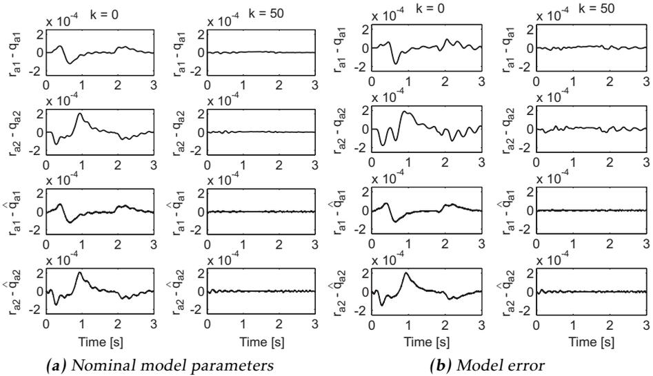
**Figure 7.7:** Case 2A: Resulting motor and joint angular position errors for ILC iteration  $k = 50$ , compared to the errors when no ILC algorithm is applied to the system (denoted  $k = 0$ ). a) nominal system parameters, b) model errors.
