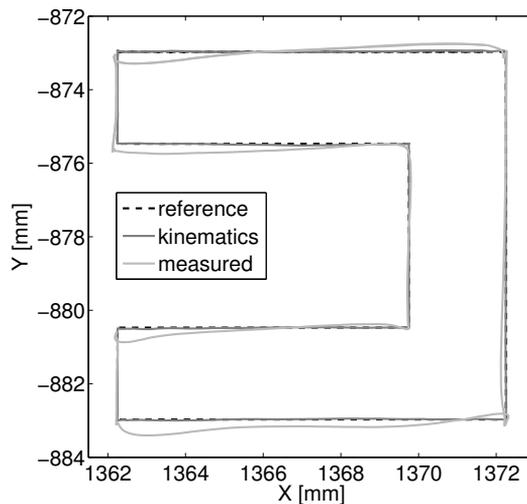
**Figure 5.14:** Tool performance after 10 iterations. The reference path (reference) is compared to the resulting path computed from the measured motor angular positions transformed by the forward kinematics (kinematics) and the measured tool position (measured).
