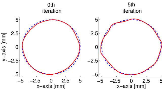
**Figure 5.10:** Measured circle of the tool when the experiment is performed with the ILC design variable  $f_c = 15$  Hz. An oscillatory behaviour is noticed for iteration 5 compared to iteration 0.
