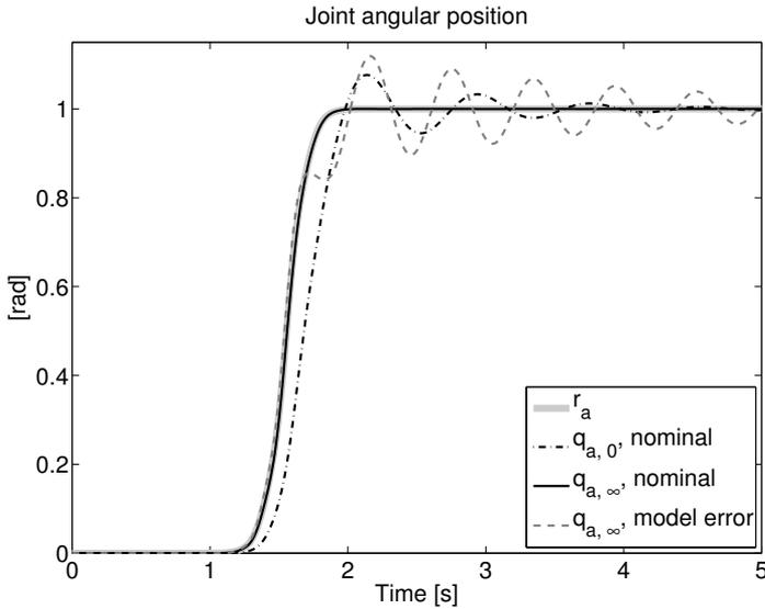
**Figure 5.18:** Resulting joint angular position when the ILC algorithm has converged (denoted  $\infty$ ). The performance is improved in the nominal case. However, when introducing model errors, the performance is deteriorated compared to when no ILC algorithm is applied (denoted 0).
