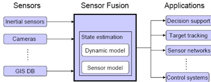
Figure 4.2: Structure of a sensor fusion system and this chapter.
