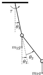
The model is a DAE whose state space form has four state variables. A reduced nonlinear model with two state variables is compared to a linear reduced model with two state variables in figure 3.1. The reduced and full order
