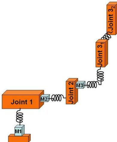
Figure 5.2: One example of an extended flexible joint model. The model has three actuated joints, two non-actuated joints, and eight degrees-of-freedom.
