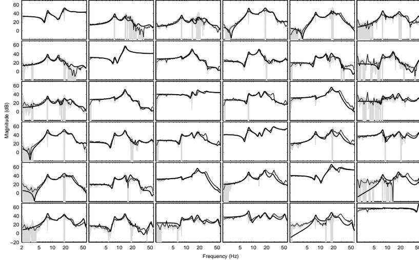
Figure 5.1: Estimated nonparametric FRF (thin line, with one standard deviation shaded) and the FRF of the resulting gray-box model (thick line) in one of the positions. Input: 6 motor torques, output: 6 motor accelerations.
