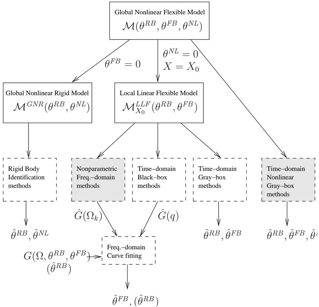
Figure 8.1: Overview of the robot identification problem and some common subproblems and identification methods. The shaded boxes denote what is treated in [4].
