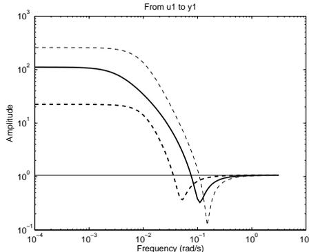
Figure 3.2: Bode plot showing the estimated output error models of the system (3.10) for a Gaussian input (thin solid) and for inputs  $u_M$  according to (3.11) with  $M = 1$  (thin dashed),  $M = 2$  (thick solid) and  $M = 8$  (thick dashed).
