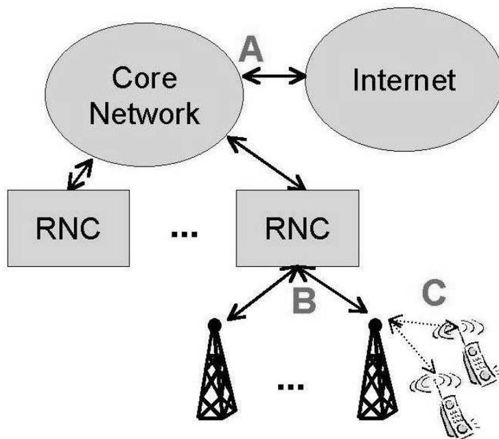
Figure 7.1: Radio network connected to a core network and the Internet
