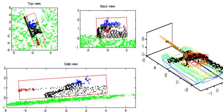
Figure 5.2: Target recognition of a tank. Left: 3D size and orientation estimation using rectangle fitting. The identified main parts are barrel (o) and turret (x). Right: Matching with low-resolution CAD model.
