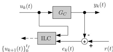
Figure 8.2: An example of a system controlled using ILC.
