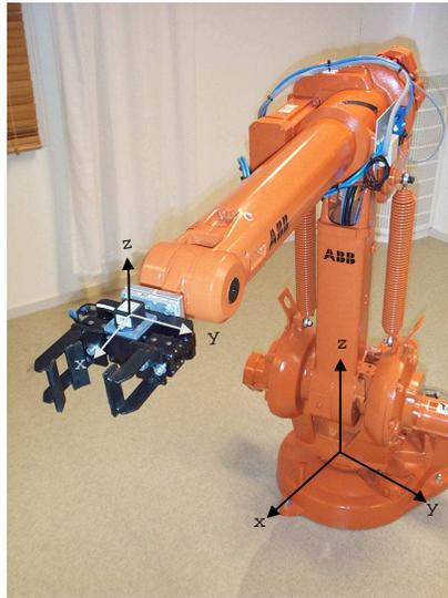
Figure 8.3: An ABB IRB1400 robot with a 3-axes accelerometer mounted on top of the gripper.
