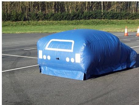
Figure 5.5: The CMBB system is evaluated in a Volvo V70 in collisions with the inflatable car on the picture.
