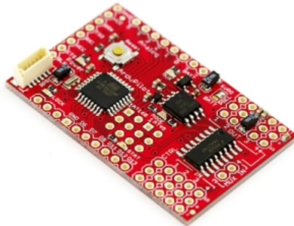
Figure 3: The ArduPilot board. Picture taken from [1]. To be able to use the board, several pins have to be soldered onto it. The white connection on the top left part of the board is used to connect the GPS.
