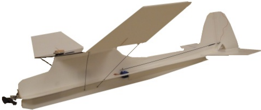
Figure 1: The plane that we use in the project. The control surfaces are rudder and elevator only.
