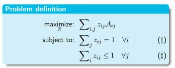
† Each measurement is associated to exactly one track/FA/NT.
