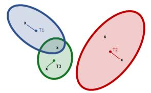
NN is a hard decision mechanism for which measurement to use for a track.
