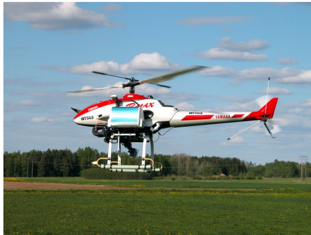
Figure 1: The Yamaha RMAX helicopter used in the collecting the data. The on-board system is equipped with an IMU (accelerometers and gyroscopes), an air-pressure sensor (barometer) and a downward looking camera. The on-board GPS receiver will be used for evaluation only.
