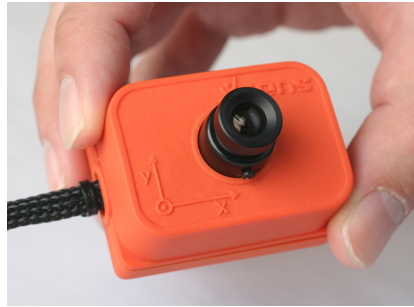
Figure 2: The combined camera and IMU sensor used to obtain the data.
