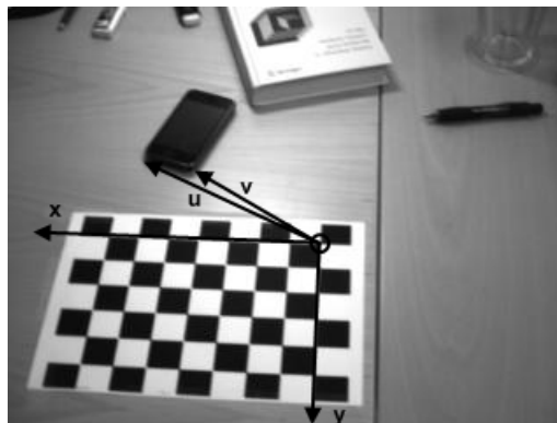
Figure 3: Position of the iPhone. The origin is indicated using a circle and the two vectors given in the figure are \mathbf{u} = (220 \quad -118 \quad 0)^T and \mathbf{v} = (151 \quad -90 \quad 0)^T (in world coordinates, unit: mm).
