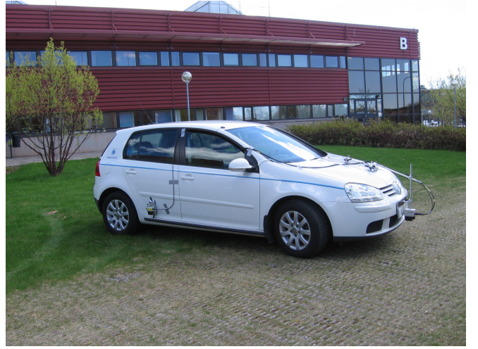
Fig. 2. The test vehicle of Linköping University is logging standard CAN data. The vehicle is in addition equipped with a GPS receiver, an IMU and an optical velocity sensor.
