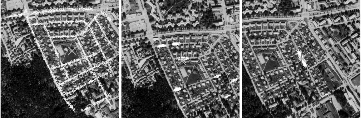
Fig. 3. Car positioning: Sequence of illustrations of particle clouds (white dots) plotted on a flight image for visualization. The center point '+' shows the true position and 'x' the estimate.
